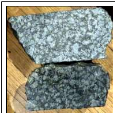
Figure 23 - Application of MATT polyurethane on lower sample
